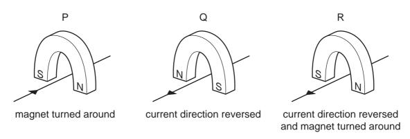
Which arrangement or arrangements will cause a force in the same direction as the original arrangement?
