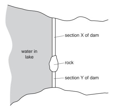
The water creates a total force on each section of the dam and an average pressure on each section of the dam.
